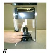
After draining all the hot water, gently scrub the sensor electrode at the nozzle end with a tooth brush and washing it well
