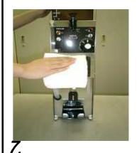
Wipe the machine with a cloth dipped in a neutral detergent solution or soap and water, then wipe it well with a dry cloth. Do not use paint thinner or other volatile fluids or alkaline detergents.
