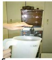
**5**. Discharge about a half of the hot water from inside through the sake drain cock into a
