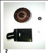
Remove the parts (Server bottle tray, Cap, Air feeder cap and filert) and wash well with hot wate.
