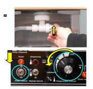
Close the Stopcock.\* (Ref. \*Note) Power switch $\rightarrow$ ON. Temp. control knob  $\rightarrow OFF$ .
