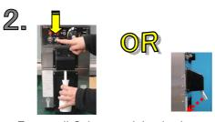
Empty all Sake remaining in the dispenser. Push the Nozzle down or dispense using the manual switch.
